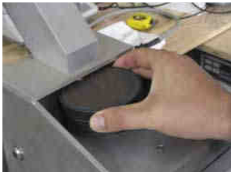
Sample being inserted on the turntable of the Blue Cube MQi Universal Spot Mineral Quantifier
